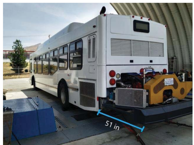
Figure 1. PHEB as tested on heavy-duty chassis dynamometer
